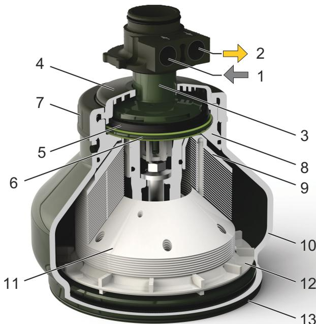
The MIB 503 section drawing illustrates the basic parts of the separator bowl
