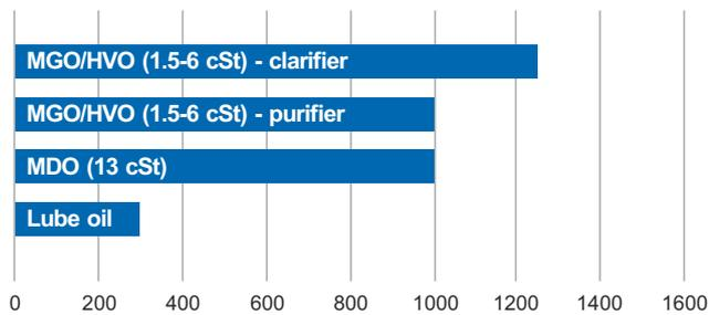
Max. recommended capacity, l/h at 40°C
